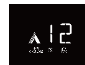
视窗放大型 windows enlarged 6.4"BND-LEDW 白色段码显示 6.4"BND-LEDW White LED segment display
